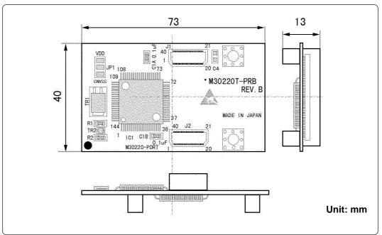
Figure 4.1 External dimensions of pod probe
